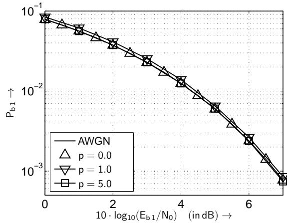
Figure 2: Bit-error-rate  $P_{b1}$  as a function of the signal- to - noise ratio  $E_{b1}/N_0$  using optimal detection (spreading sequences  $\mathbf{b}_1 = (+1, +1, +1)^T$  and  $\mathbf{b}_2 = (+1, -1, +1)^T$ )
