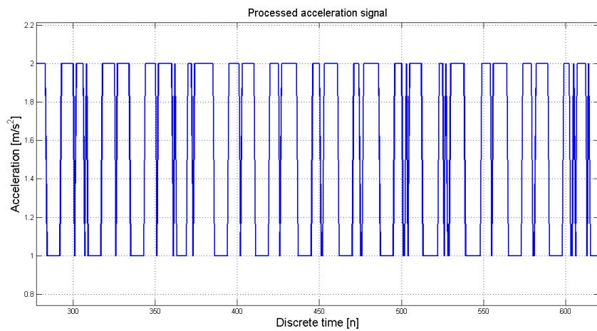
Figure 2: Acceleration signal with applied threshold.
