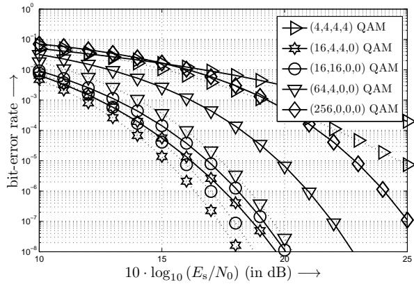
Figure 2: BER with equal-SNR PA (dotted line) and without PA (solid line) when using the TMs listed in Tab. 1 and transmitting 8 bit/s/Hz over frequency selective channels with  $L_c = 4$ .
