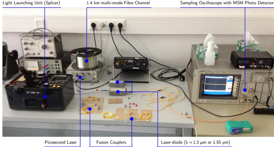
Figure 3: Measurement setup for determining the MIMO specific impulse responses.
