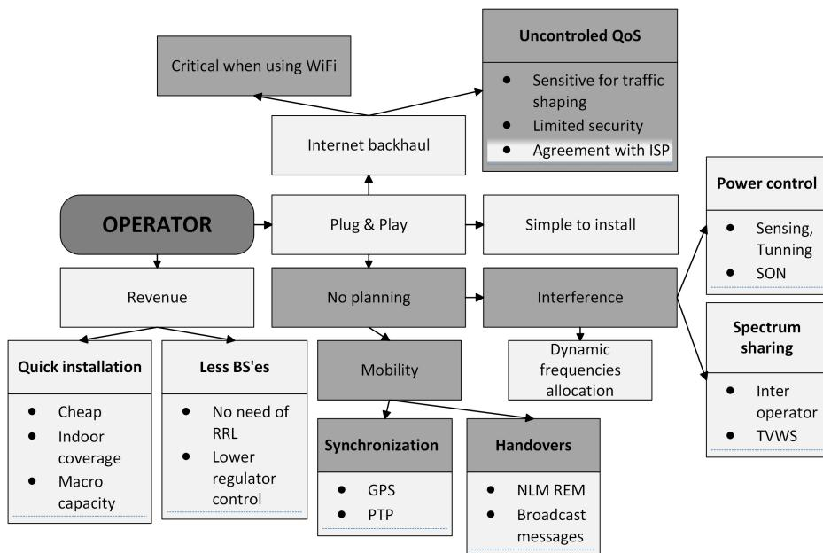
**Figure 1:** Advantages and disadvantages of HNB from the operator point of view. Note that light grey colour in the figure shows advantages of HNB and dark grey colour refers to disadvantages (RRL here refers to the Remote Radio Links, PTP – Precision Time Protocol, ISP – Internet Service Provider, and SON - Self-Optimizing Networks).
