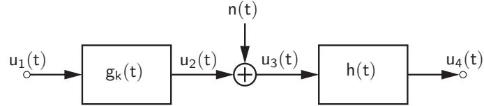
Figure 5: Transmission system model.
