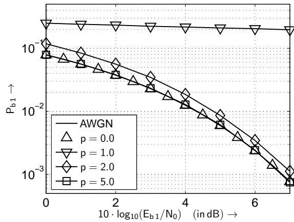
Figure 3: Bit-error-rate  $P_{b1}$  as a function of the signal-to-noise ratio  $E_{b1}/N_0$  using optimal detection (spreading sequences  $\mathbf{b}_1 = (+1, +1, +1)^T$  and  $\mathbf{b}_2 = (+1, +1.1, +0.89)^T$ )
