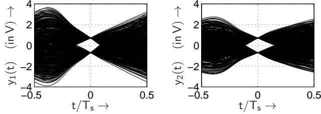
Figure 14: Eye diagram patterns of both received signals when applying zero-forcing equalisation.
