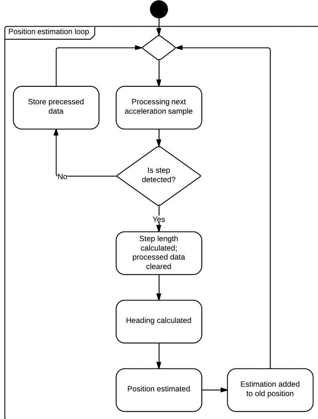
Figure 7: Low power algorithm structure.
