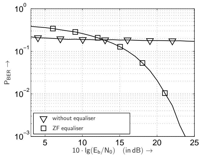
Figure 15:  $(2 \times 2)$  MIMO BER probability as a function of bit energy  $E_b$  to noise PSD with and without applying the zero-forcing equalising method using the deconvolved MIMO impulse responses at 1576 nm operating wavelength and transmitting with a bit rate of 1.24 Gb/s.
