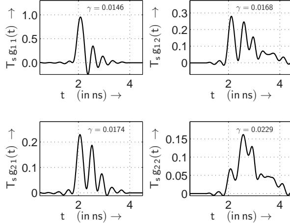
Figure 12: Deconvolved measured electrical MIMO impulse responses with respect to the pulse frequency  $f_T = 1/T_s = 620$  MHz at 1576 nm operating wavelength using the regularisation filter function with  $\gamma$  values according to the Gans' criterion.
