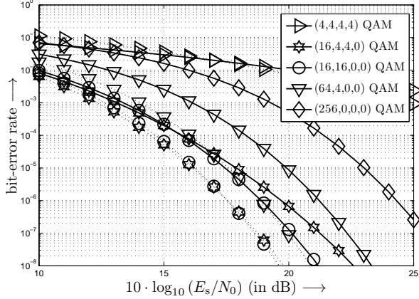
Figure 1: BER with equal-SNR PA (dotted line) and without PA (solid line) when using the TMs listed in Tab. 1 and transmitting 8 bit/s/Hz over frequency selective channels with  $L_c = 1$ .
