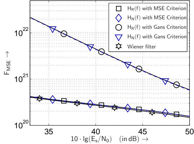
Figure 9: Quality  $F_{\text{MSE}}$  of the deconvolved impulse responses as a function of signal energy to noise power spectral density using different filters.
