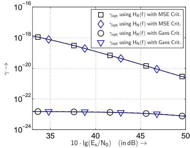
Figure 10: Choice of optimal  $\gamma$  when filtering with the regularisation filter  $H_R(f)$  and the Nahman-Guillaume filter  $H_N(f)$  minimizing the MSE and using the Gans' criterion.
