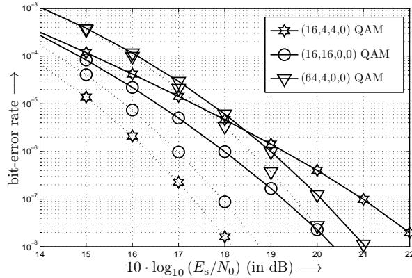
Figure 4: BER with equal-SNR PA when using the TMs shown in bold in Tab. 1 and transmitting 8 bit/s/Hz over frequency selective channels with  $L_c = 4$  (dotted line) as well as frequency non-selective channels (solid line).
