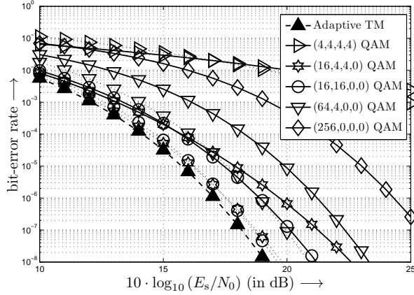
Figure 3: BER with equal-SNR PA (dotted line) and without PA (solid line) as well as adaptive choice of the TM combined with equal-SNR PA (dashed line) when using the TMs listed in Tab. 1 and transmitting 8 bit/s/Hz over frequency selective channels with  $L_c = 1$ .
