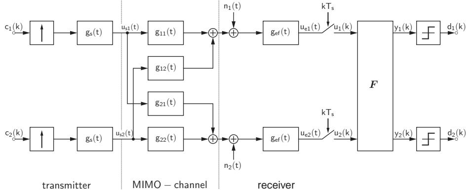
Figure 13:  $(2 \times 2)$  MIMO baseband transmission system model with discrete zero-forcing equaliser.
