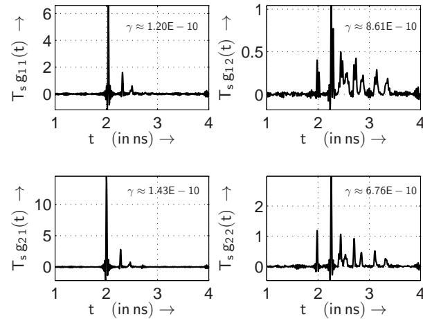
Figure 11: Deconvolved measured electrical MIMO impulse responses with respect to the pulse frequency  $f_T = 1/T_s = 620$  MHz at 1326 nm operating wavelength using the regularisation filter function with  $\gamma$  values according to the Gans' criterion.
