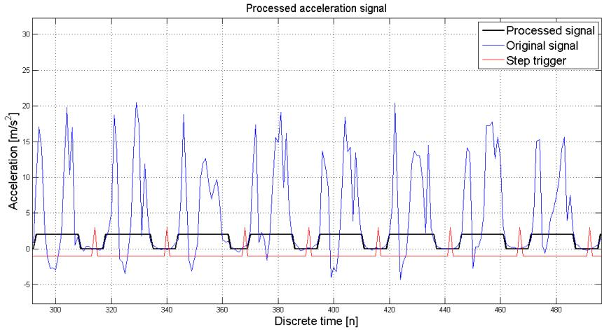
Figure 8: Step detection in acceleration signal.
