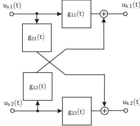
Figure 4: Electrical MIMO system model (example:  $n = 2$ )
