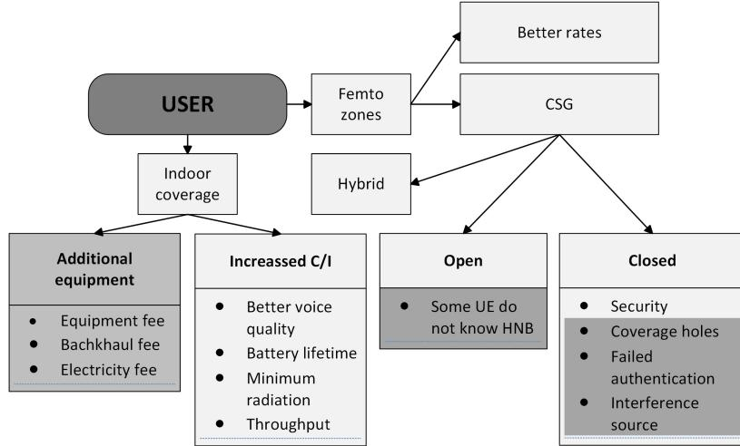
**Figure 2:** Advantages and disadvantages of HNB from the user point of view. Note that light grey colour in the figure shows advantages of HNB, dark grey colour refers to disadvantages (CSG here refers to the Closed Subscriber Group).
